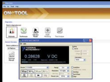
Diagnostic device readouts, like the integrated Built-In Test Equipment (BIT/BITE) interfaces, are accessible via ONeTOOL.
